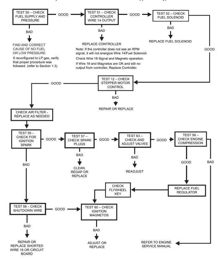
IMPORTANT NOTE: Clear any faults in the controller before proceeding with any running diagnostic steps!
