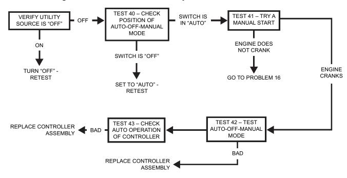
Problem 16 – Engine Will Not Crank When Controller Switch is Set to MANUAL or Controller Goes Dark and Reboots
